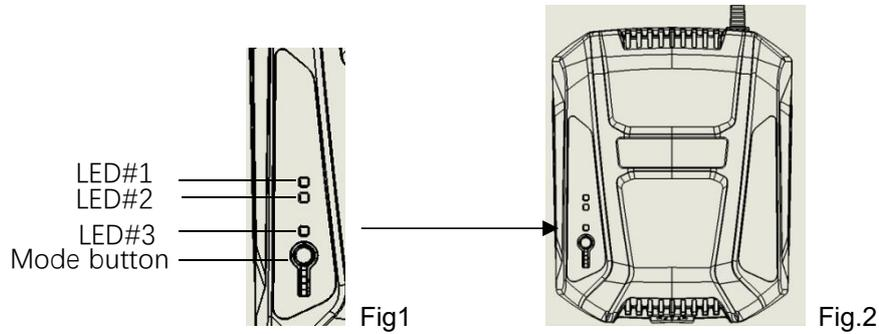
**LED INDICATORS:** Indicate the charging status. There are three LEDs.: #1 LED indicates standard charging, #2 LED indicates abnormal charging, and #3 LED indicates a fast charging.
